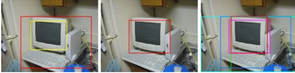
Figure 5.2: Detection results from NMS (red line in left) and subset optimization (center). Bounding boxes (BB) (right) represent the highest confident proposals got from different steps (blue BB: CNN, green BB: maskout, pink BB: re-train, cyan BB: MIL). We compare the detection results by bounding boxes in different colors, which shows our re-training strategy is able to get the denoising proposals by re-weighting object proposals according to the detection scores and the overlap ratios of the proposals.
