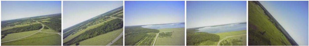
Figure 4.8: Illustration of samples from the UAV flying dataset. The UAV flies with large variations of orientation. The horizon line is always recognizable and provides reference for UAV orientation.
