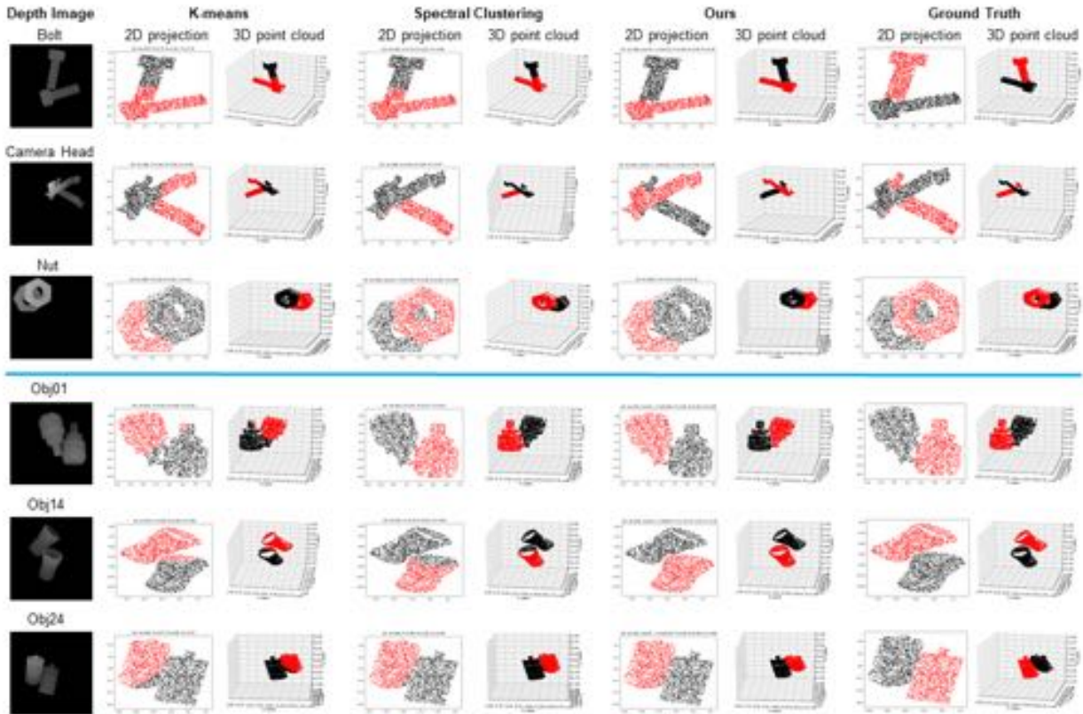
Figure 4.4: The qualitative results of instance segmentation of 2D projection and 3D point clouds with N = 2 instances.
