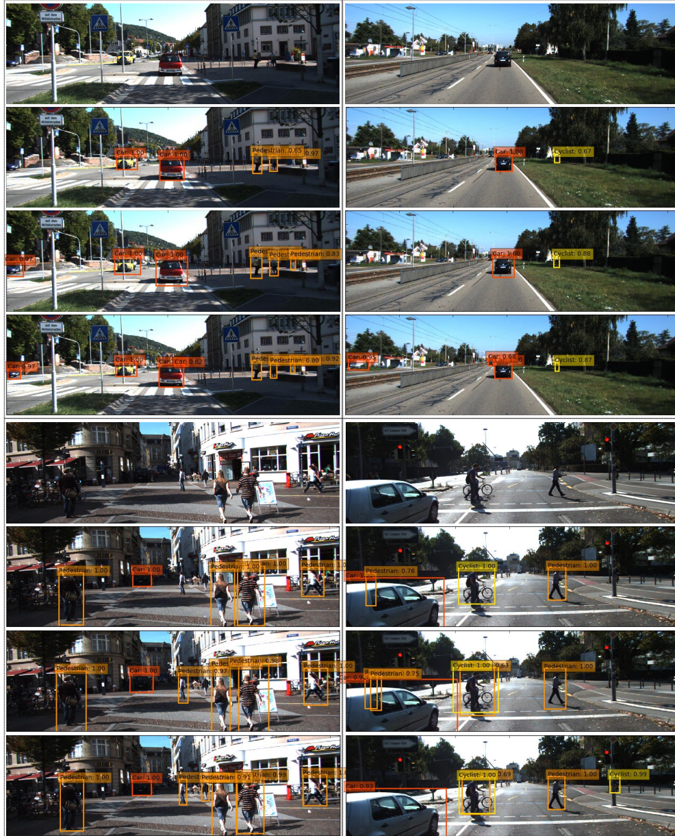
Figure 3.7: Four sets of comparative detection examples of SSD and MDFN on KITTI dataset. In each set, the four images, from top to bottom, represent the original image and the results from SSD, MDFN-I1 and MDFN-I2 respectively.
