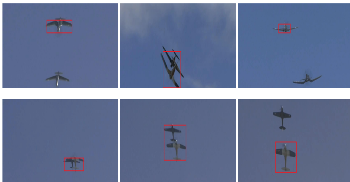
Figure 4.15: Frames showing our tracker narrows down to the prime object in a scene once the multiple objects are at a suitable distance apart or one of the objects move out of scene.
