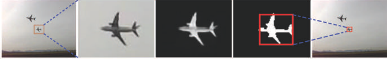
Figure 4.4: Refinement process: (From left to right) Selected region around the prime object based on the peak value for the refinement process (brown bounding box), the chosen area for refinement (zoomed in for better view), saliency map generated for the chosen area, post-processed binary image, prime salient object re-detected (notice the change in the size bounding box before and after the refinement process) to update the tracker.
