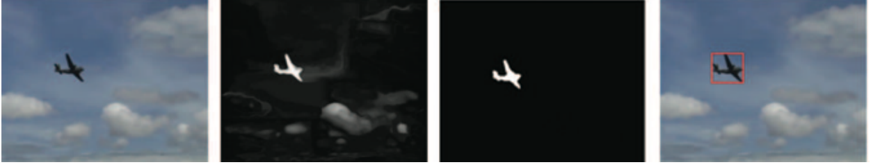
Figure 4.3: From left to right: Original frame, generated saliency map, binary image and the object boundary using our object detection technique.
